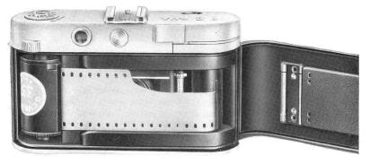
The illustration above shows the correctly loaded camera before closing and setting the film counter. The rewind knob is pushed down into the body, and the film lies flat in the film track. Now close down the camera back, and press it against the body; make sure that the back lock engages properly.
