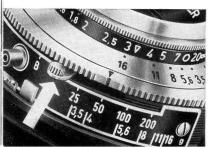
until the red index line is above the required exposure time. When set to "B" the shutter remains open as long as the release button is depressed.
