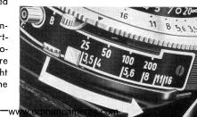
The Prontor-SVS shutter with exposure value scale carries shutter speeds from 1 to 1/300 second, as well as a "B" setting for time exposures. It is MX-synchronized for flash (see pages 24 to 27). For all shots without flash it is immaterial whether the synchronizing lever is set to M or X.
